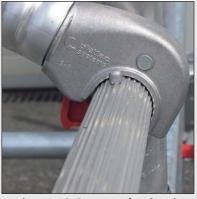
A characteristic aspect for the plettac alu star series is the aluminium die casting claw for the quick and effective combination of ladder frames with guard rails and diagonals. The improvement makes erection and dismantling much easier and reduces assembly times. The steps of the ladder frames are manufactured with special profiled nonskid tubes and are used for interior access.
