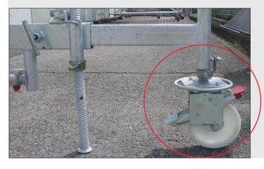
Only one castor for all plettac aluminium rolling towers independent from the erection height. The enables the castor 11.9 kN with a wheel diameter of 200 mm. The high quality castor with double break action increases the stability of the rolling tower.
