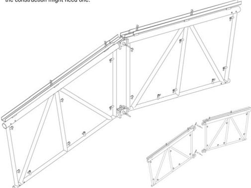
The structural stiffness of main and make-up trusses is realized by transverse frames secured to the parallel modular beams. SL Diagonals and guard rails to the lower chord are required according to the length of the trusses. For all connections of transverse frames, diagonals and guard rails the modular beams are equipped with gravity pins.
