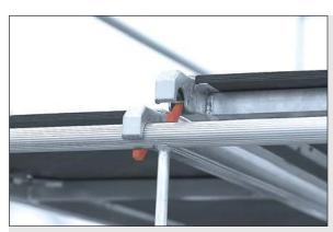
Clever assistance during the dismantling process. The rapid locks of the assco rapido decks and access decks allow to lean the deck to the top of the ladders steps at one side without falling into secured postion immediately. One man is able to dismantle the deck in case of necessity.
