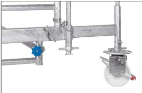
The telescopic mobile beam is a safe foundation used with greater assembly heights. The adjustable spindle assures the horizontal position also for extending the telescopes. Telescopes of assco rapido mobile towers are secured and fixed without the need of tools.
