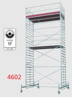
Do you have to handle bulky equipment or do you need a wider working space? The aluminium assco rapido mobile tower 4602 provides a working area of 1.50 m width and 2.85 m length. The max. working height is 9.60 m in the open and 13.60 m inside closed areas. Using this type of scaffolding you will need the mobile beam for working above 7.50 m only. The height- adjustable castors are easily fit into the tubes of the ladder frames and secured by wing bolts.
