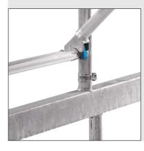
The assco rapid locking system for decks, braces and guard rails are long lasting and robust with their casting housings from aluminium held in position and secured by spring loaded in steel reinforced fingers from polyamide. Colour coding of the fingers allows an easy separation between braces and guard rails - without measuring. The steps of the ladder frames are manufactured with special profiled nonskid tubes and are used for interior access.
