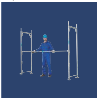
Assemble vertical frame and secure with guard rail
